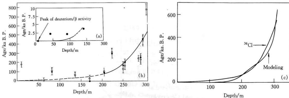
Fig. 2 Dating of the Guliya ice core. (a) Stratigraphy. The black circles represent  $^{14}\text{C}$  dating, the solid line is the dust layer curve, and the dashed line is the modeling curve. (b)  $^{36}\text{Cl}$  method. The black circles are  $^{36}\text{Cl}/\text{Cl}$ , and open circles are  $^{36}\text{Cl}/\text{g}$ . (c) Modeling method; showing the calculated result of the ice-flow model based on equation (1).
