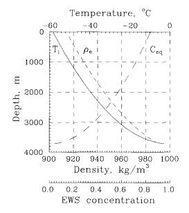
Fig. 4. Calculated temperature of ice  $(T_i)$ , density  $(\rho_e)$ , and concentration  $(C_{eq})$  of EWS in the borehole.
