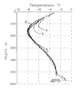
Fig. 5. Temperature distribution in the Austfonna borehole: (a, b, c) measured after break of drilling on respective depth; (d) measured after input of additional ethanol to the borehole.
