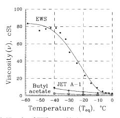
Fig. 3. Viscosity of EWS at equilibrium temperature compared with JET A-1 and butyl acetate.
