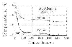
Fig. 6. Time-scale variation of the temperature in the Austfonna borehole.
