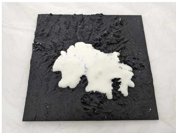
Photo 1. Flubber placed on a 3D-printed model of a mountain landscape flows downhill, analogous to how glaciers flow.
